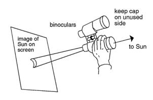
However, **take note**, when projecting you can easily burn out the optics in your telescope of you are not careful. There are two things to watch for; both relate to the intensity of the image at the prime focus of your telescope. This will be very hot -- brighter than sunlight
