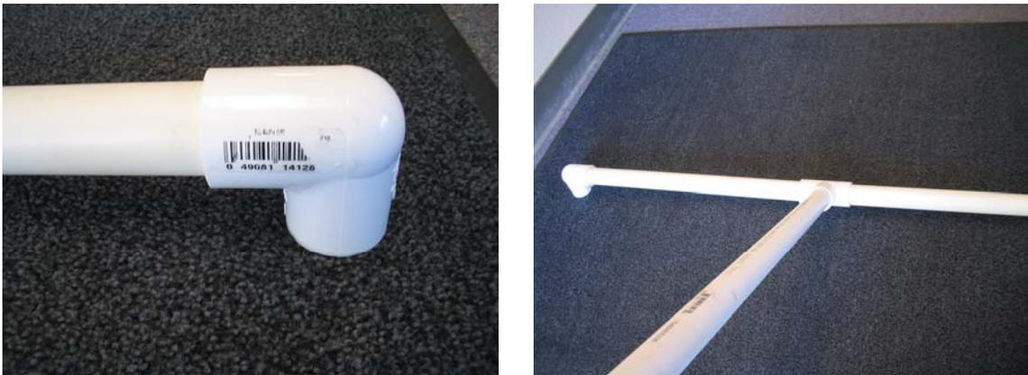
*Place the 4 elbow connectors on the open ends of the base you created. Now your antenna will stand upright and off the ground.*
