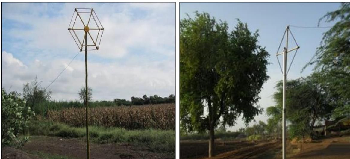
**Fig. 3:** Loop Antenna: (a) Hexagonal Loop Antenna (b) Square Loop Antenna.
