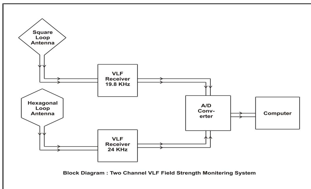
**Fig. 1:** Block Diagram of VLF Field Strength Monitoring System which Consists of Loop Antennas, SID Monitor, A/D Converter and Computer.
