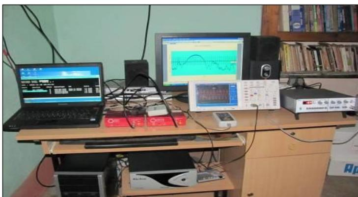
**Fig. 2:** Experimental set up—Two Channel VLF Field Strength Monitoring System.
