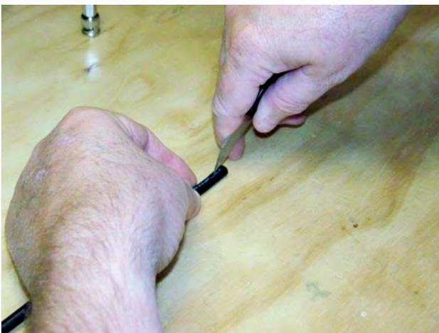
From the first cut around the cable, take the knife and cut a line to the end of the cable.
