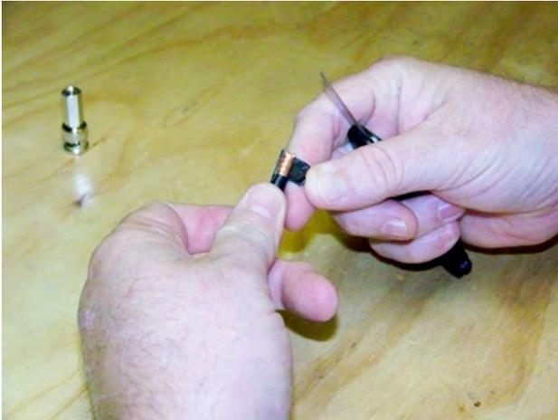
Remove the outside cover from the inner wires. You will now see the copper shielding.
