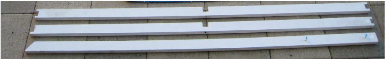
1. Horizontal Arm (*top*): has "bridle" cuts on both ends to hold the wires and a "cross lap" cut in the middle to be joined with the Vertical Arm.
