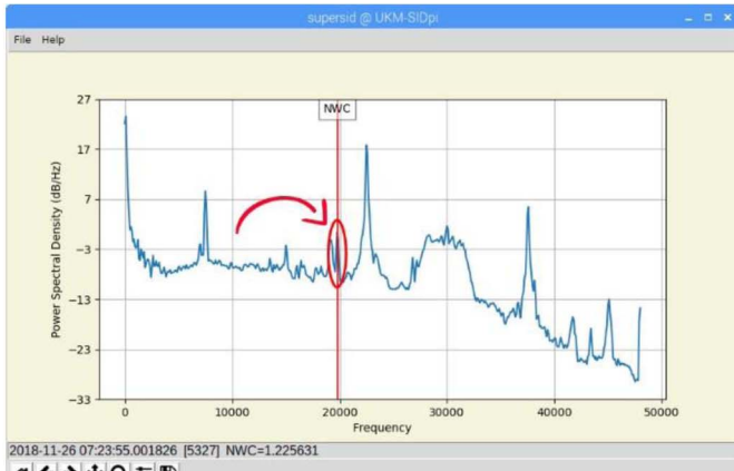
Fig. 11. Clear peak of 19.8 kHz detected by the UKM-SID \pi system
