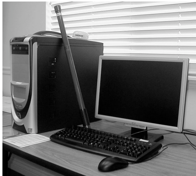
Figure 1. Typical beacon monitor consisting of a Linux PC with a PCI-based software radio installed. The GPS receiver is sitting on the PC case, and the wideband active antenna is leaning against the PC. The GPS receiver and active antenna are installed outdoors at roof level when the monitor is deployed.
