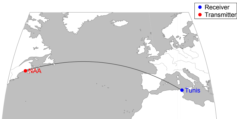
Fig. 1. Great Circle Path (GCP) between the NAA transmitter (24 kHz) and receiver at Tunis over a distance of \sim 6326 km.
