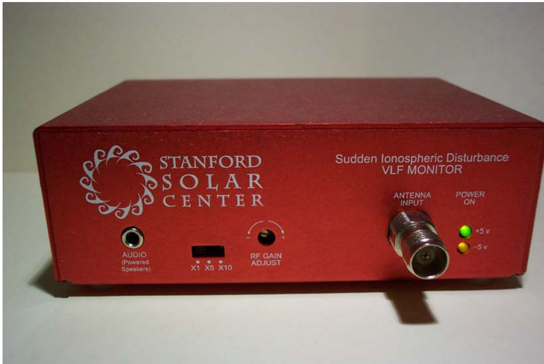
Sudden Ionospheric Disturbance (SID) Monitor
