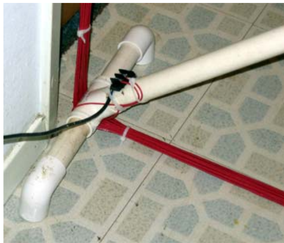
Note the use of zip ties to make sure the wire windings stay together.
