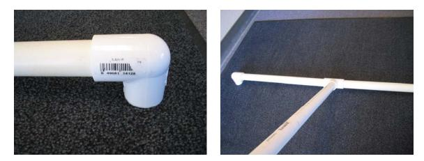
Place the 4 elbow connectors on the open ends of the base you created. Now your antenna will stand upright and off the ground.
