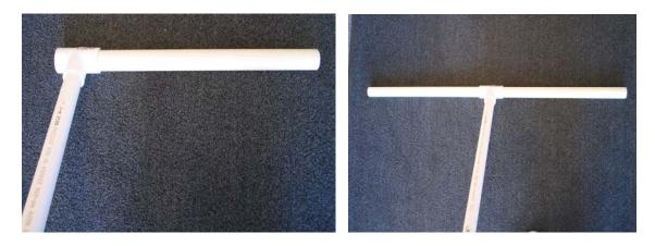
Standing your antenna up, place one of the smaller lengths of PVC pipe in each end of the T connector. **Repeat** this on the other side of the frame that touches the ground.
