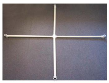
Turn your end connectors so the openings are perpendicular to the 4 way hub (as shown). This is the completed frame, you can work with this design to create "feet" as we did, or affix it to a mast. Mast design examples can be seen in appendix E and also on our website: <a href="http://solar-center.stanford.edu/SID/antenna\_designs.html">http://solar-center.stanford.edu/SID/antenna\_designs.html</a>
